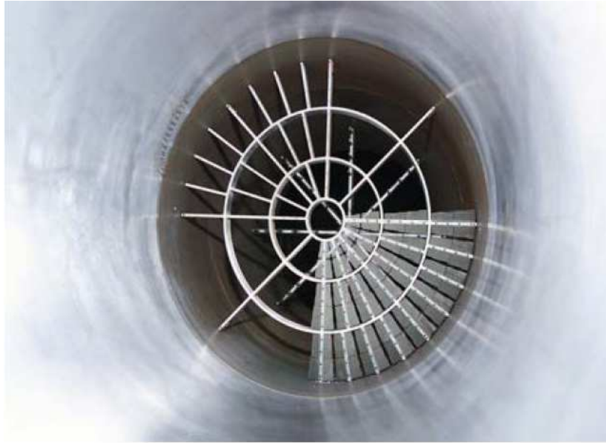
Figure 2.20: Sample of a modern distortion screen with varying vane sizes and densities. Image courtesy of Arnold Engineering Development Center[58].
