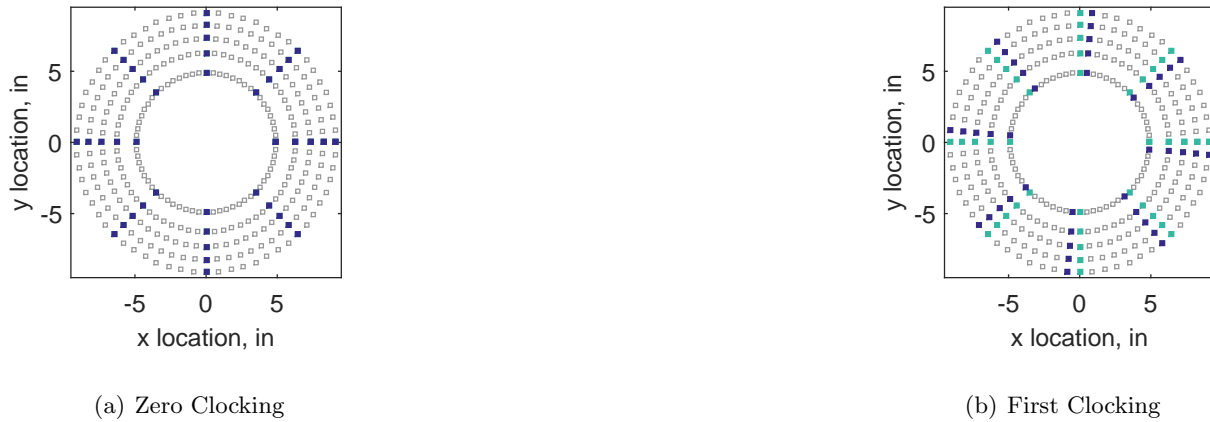
Figure 5.1: Clocking example of the 40 probe subset, with the darker color representing the clocking.
